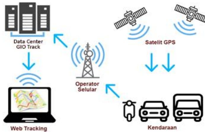
Gambar 2.2 Cara Kerja *Global Positioning System*
