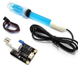
Gambar 2.9 sensor pH kit [16]
