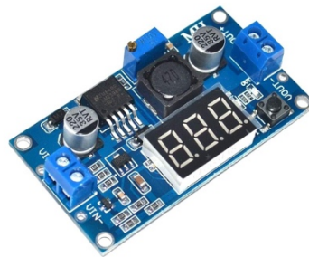
Gambar 2. 13 DC StepDown Converter
