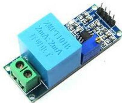
Gambar **Error! No text of specified style in document.**4 Sensor ZMPT101B
