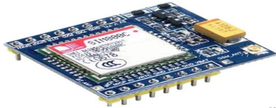
Gambar 2. 12 Modul GSM SIM 800C [30]
