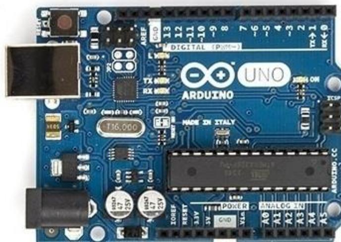
**Gambar 2.1 Board Arduino Uno**
