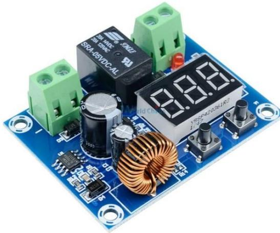
Gambar 2.30 Low Voltage Disconnect (LVD)
