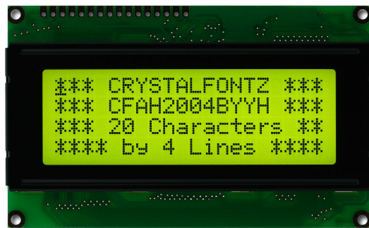
Gambar II.4 LCD 20 kolom 4 baris
