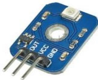
Gambar 2.6 Sensor Ultraviolet
