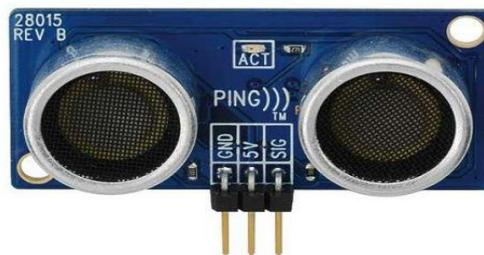
**Gambar 2.7** Sensor ultrasonik PING
