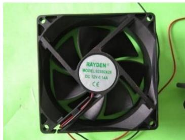
**Gambar 2.17 Fan DC/Motor DC**
