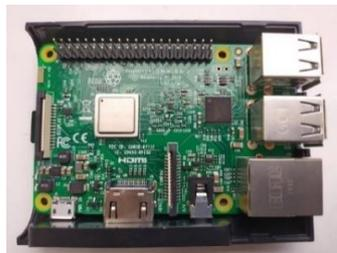
**Gambar 2.12 Raspberry Pi 3 Model B**
