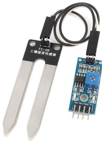
**Gambar 2.3 *Soil Moisture Sensor* [12]**
