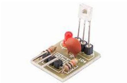
**Gambar 2. 3 Sensor *Laser Detector***
