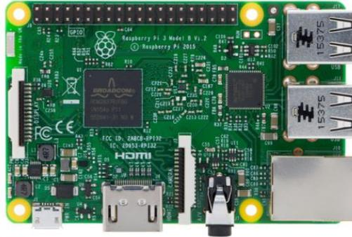
Gambar 2.7 Raspberry Pi 3 Model B [10]
