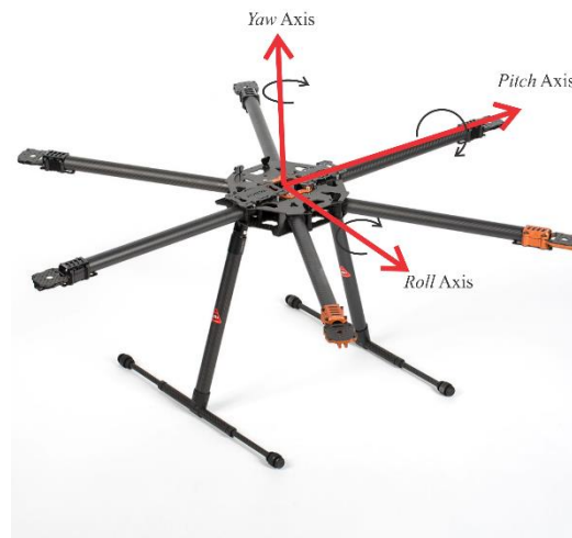
Gambar 2. 2. Tiga sumbu kendali dinamika gerak hexacopter [6]
