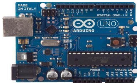
**Gambar 2. 1 Board Arduino UNO** <sup>[13]</sup>
