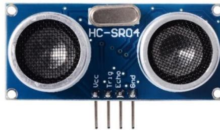
**Gambar 2.7 Sensor Ultrasonik**
