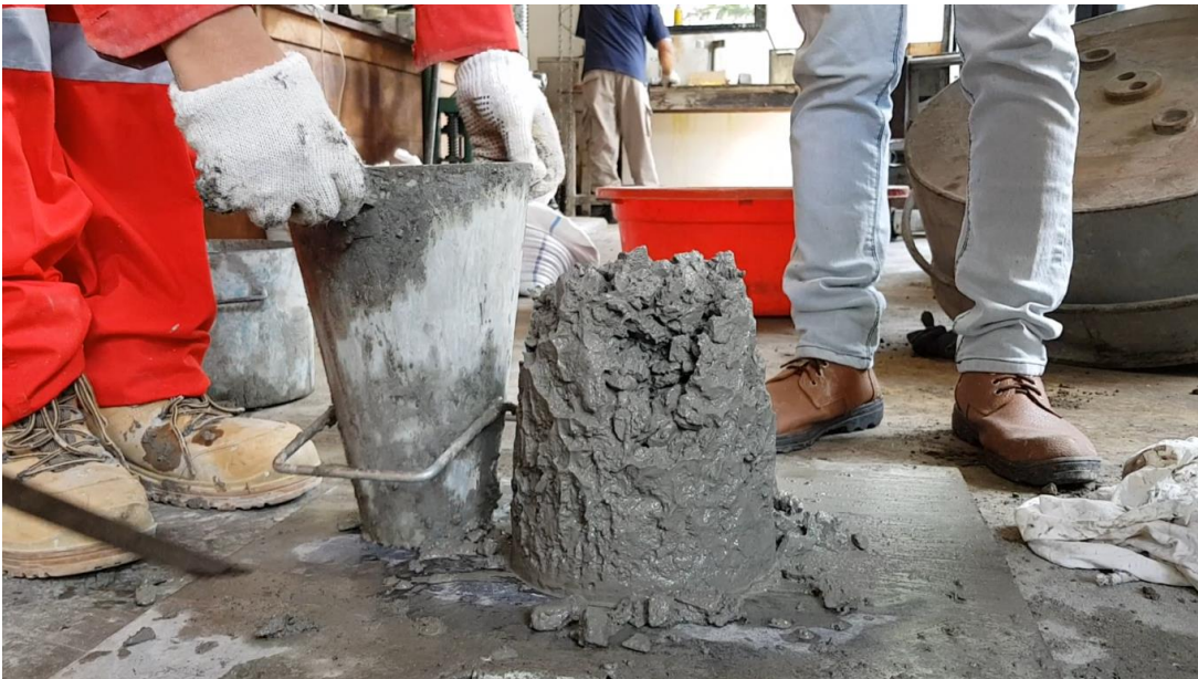
Gambar 4. 5 Proses Uji Slump
