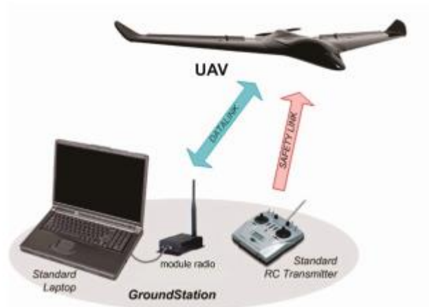
Gambar 2.1 Ilustrasi Ground Control Station [6]
