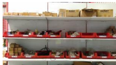
Picture 7. Set In Order In The Placement Of The Size Small Spare Parts
