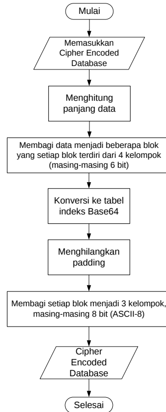
Gambar 7. Flowchart Algoritma Decoding Base64
