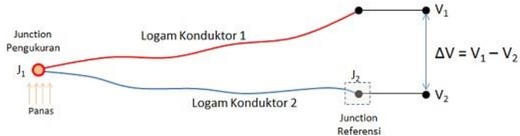
Gambar 2.20 Prinsip kerja Thermocouple [9]
