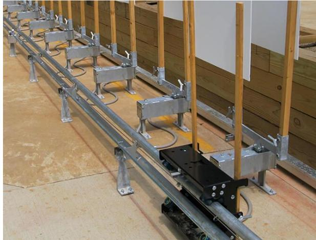
*Gambar 26. Moving Target Track*
