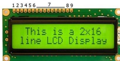
*Gambar 2.5 LCD 16x2*
