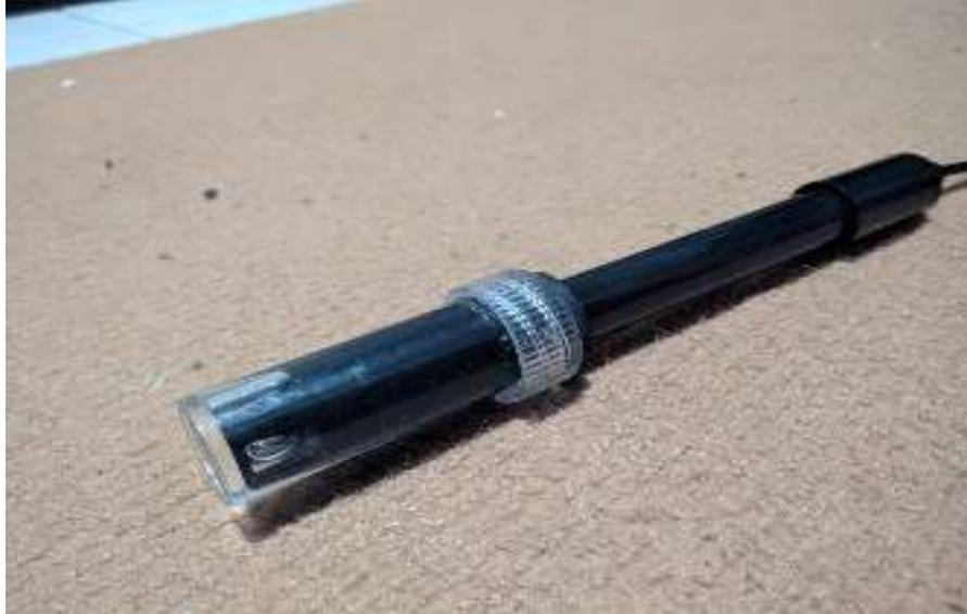
**Gambar 4. 5 Sensor pH E-201-C**
