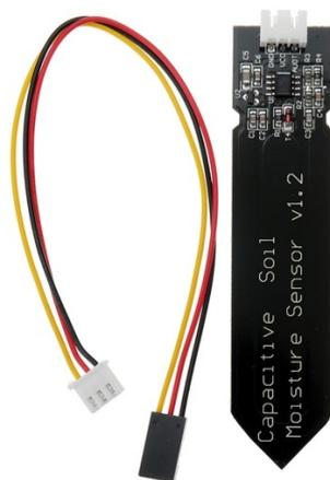
**Gambar 2.23** *Sensor Soil Moisture* [12]
