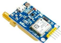
**Gambar II.9 Sensor GPS**
