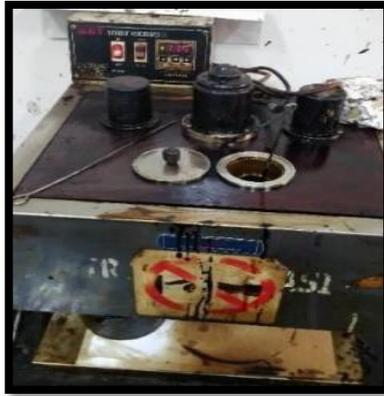
**Gambar 2.6 Saybolt Viscometer**
