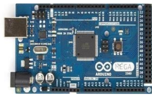
Gambar 2.1 Tampilan Arduino Mega2560
