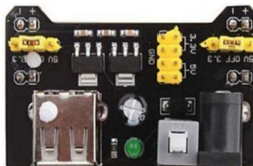
Gambar 2.5 Tampilan MB102 Breadboard Power Suply
