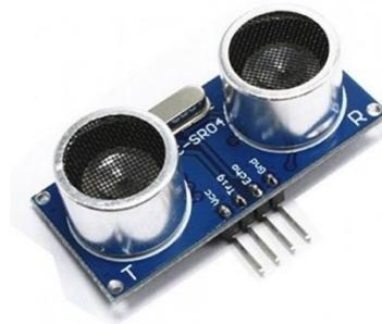
Gambar 2.3 Sensor Jarak Sensor Ultrasonik
