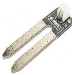
Gambar 2.7 Sensor Soil Moisture YL-69
