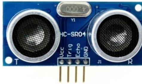
Gambar 2. 12. Sensor ultrasonik HC-SR04
