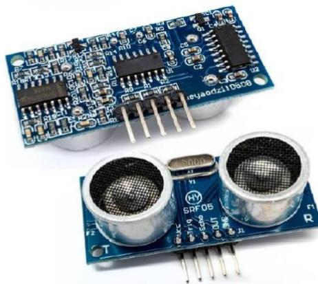
**Gambar 2.2 Sensor Ultrasonik HY-SRF05**
