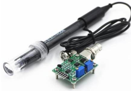
**Gambar 2.8** Sensor PH-4502C.
