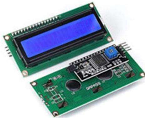
**Gambar 2. 14** LCD 16 x 2
