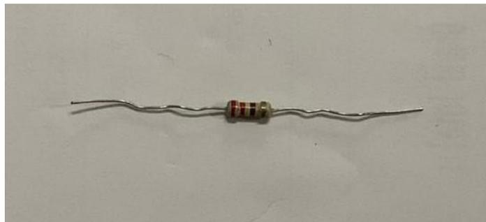
Gambar 2. 1 Fixed Resistor Non-SMD
