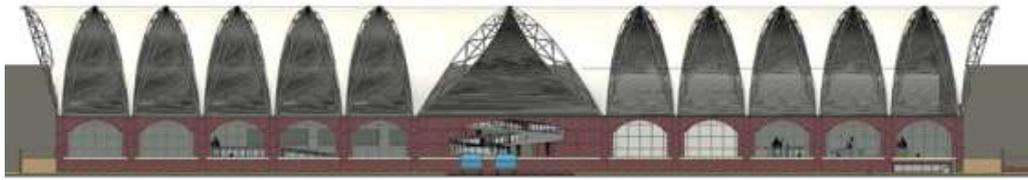
**Gambar 5. 44 Material Atap Membrane**
