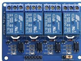
Gambar 2.8 Tampilan Relay 4 Channel
