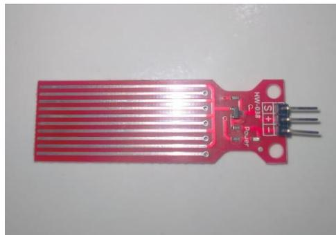
Gambar 2.7 Sensor Water Level
