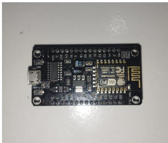
Gambar 2.17 NodeMCU ESP8266
