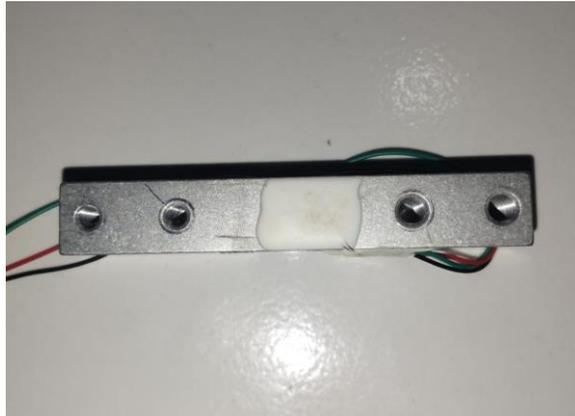
Gambar 2.5 Sensor Load Cell
