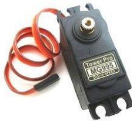
Gambar 2.16 Motor Servo MG955
