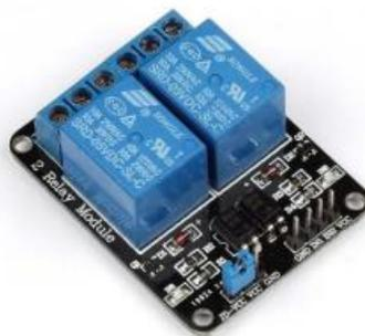
Gambar 2. 5 Module Relay 2 Channel
