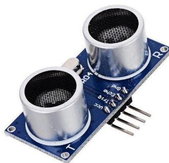
*Gambar 2. 6 Sensor Ultrasonic*
