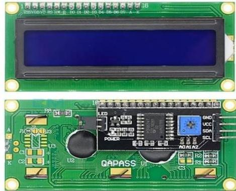
Gambar 2. 4 LCD 16X2 I2C
