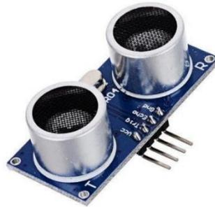
Gambar 2.3 Sensor Ultrasonik
