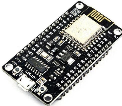
**Gambar 2.4** NodeMCU ESP8266.
