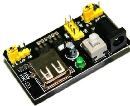
Gambar 2. 7 Tampilan fisik power supply MB102
