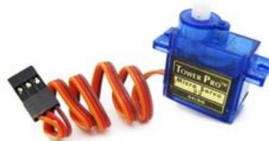
Gambar 2.5 Motor Servo Sg90
