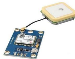
Figure 2 GPS Module 6m Ublox Neo V2
