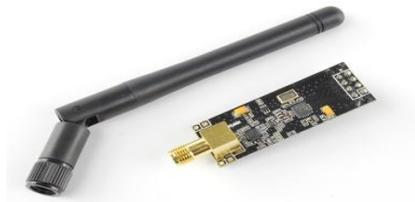
Figure 3 Module NRF24
