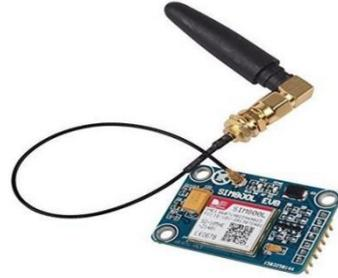
Figure 4 Module SIM800L
