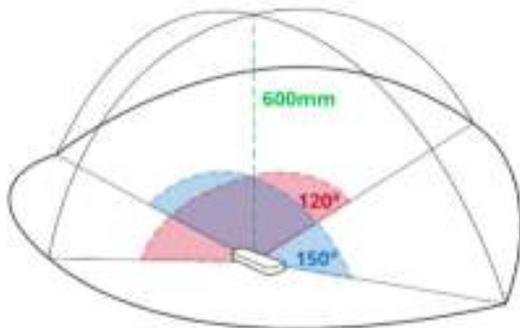
Figure 1. Area Coverage Leap Motion Controller
