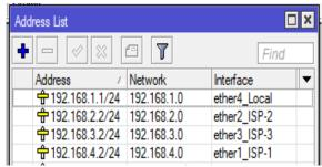
Figure 4 IP Address Configuration
