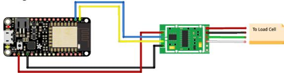
Figure 3. Communication NodeMCU and Load Cell
