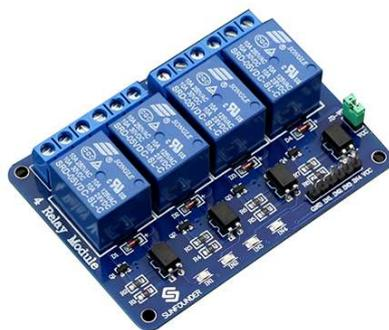
**Gambar 2-16. Relay 4 Channel**
