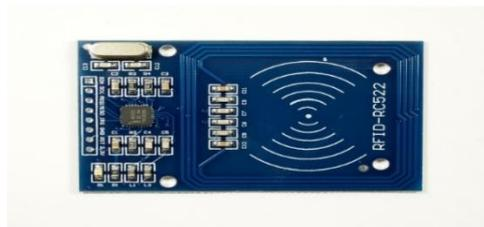
Gambar 2.10 Mifare RC522 RFID Reader Module
