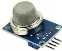
Gambar 2.9 Sensor Gas MQ-135
