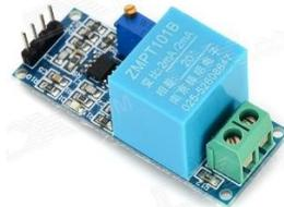
Gambar 2.5 Sensor Tegangan ZMPT101B
