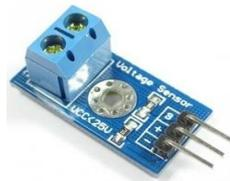
Gambar 2.6 Sensor Tegangan DC
